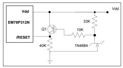
Fig. 5-35 Residue Voltage Protection Circuit 1
